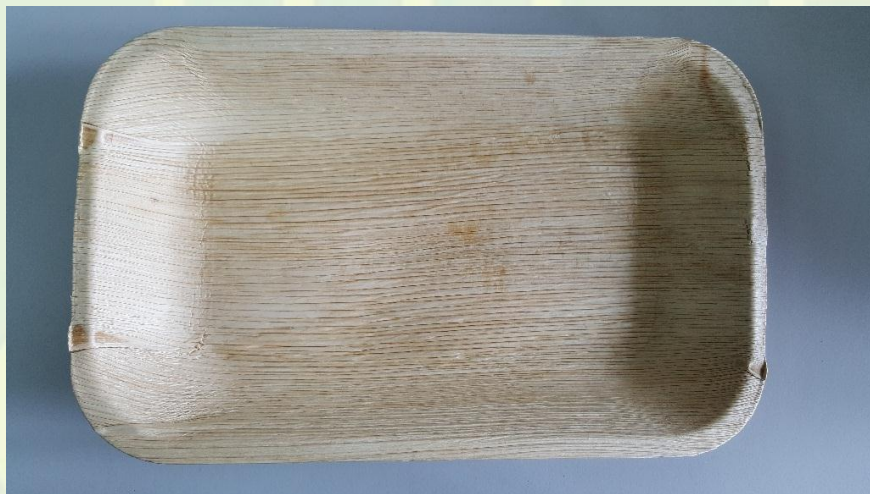
Figure 5. Photograph of 'Biomass Based Products for Food-Contact Applications; Trademark: Fallaleaf' Sample after Acid Resistance Test
